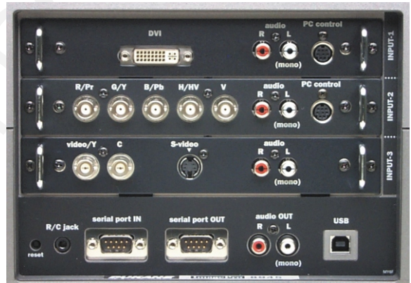
The ImagePro 8945 input modules are easily accessible.
